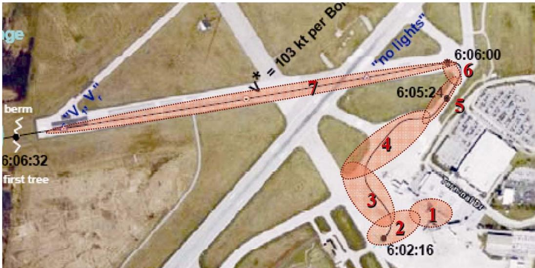
**Photo 2: Accident Aircraft Flight Segments**
