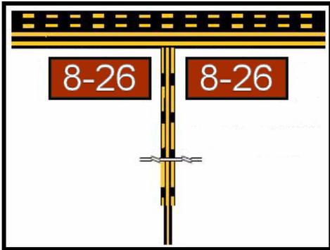
**Figure 4: Enhanced Hold Short Marking with Surface Painted Holding Position Signs**
