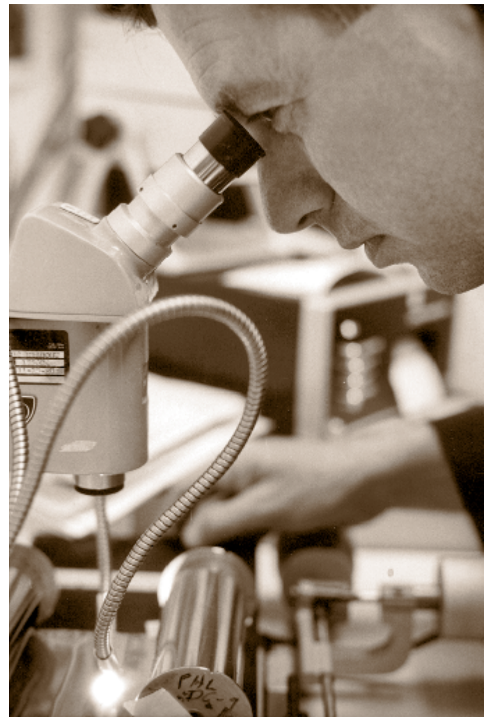
An ALPA accident investigator uses a special microscope to examine foil tape from the flight data recorder retrieved from an accident circa 1978.
