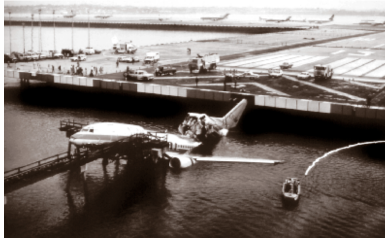
The crash of USAir Flight 5050 resulted from a high-speed rejected takeoff at New York’s LaGuardia Airport in September 1989. Investigation into the accident led to improved FAA regulations covering rudder trim systems in the B-737-300/-400/-500, the B-767, the B-757, and the B-747-400.
