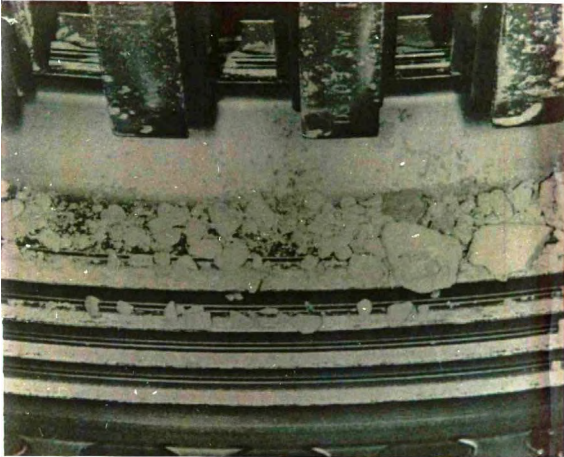
Figure 7 Accumulation of Ash in the HPT Rotor
