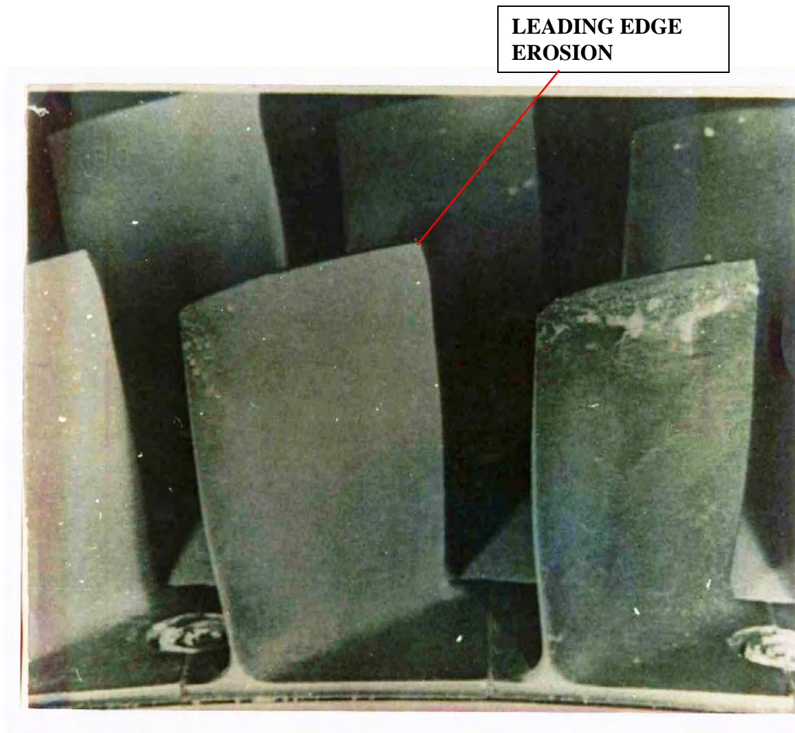
Figure 9 HPC Blades Leading Edge and Tip Erosion
