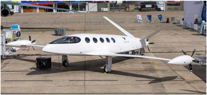
An electric-powered Eviation Aircaft "Alice" prototype, expected to enter commercial service in 2022.
